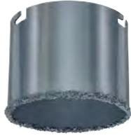
Holesaw, tungsten carbide gritted, precision formed body, coated with special tungsten carbide grit, high temperature brazed, for aerated concrete blocks, masonry, tiles, ceramics, natural stone, lightweight building materials, plasterboard and plastics, for installation work eg fitting switches, sockets and pipes.
