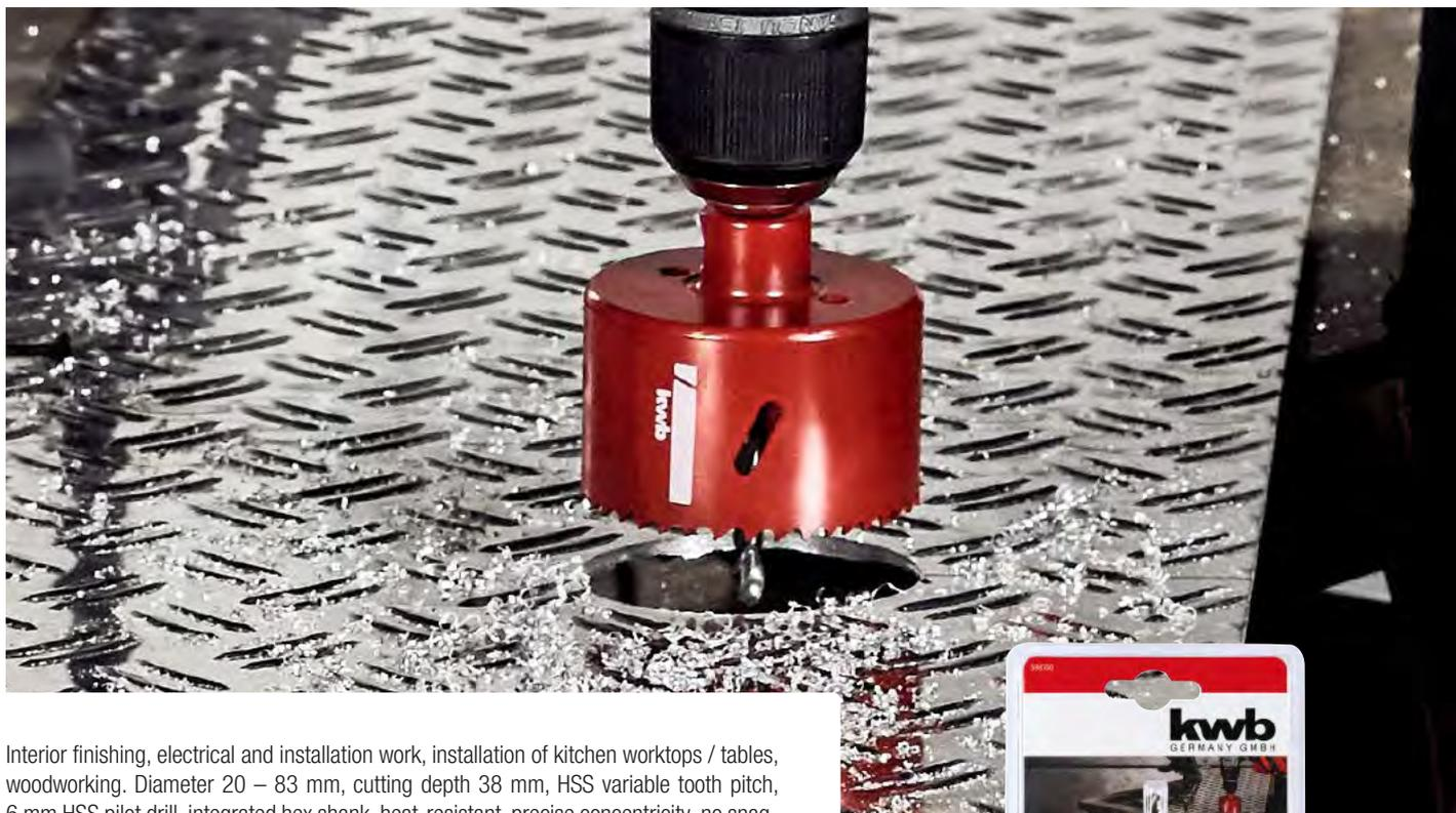
Interior finishing, electrical and installation work, installation of kitchen worktops / tables, woodworking. Diameter 20 – 83 mm, cutting depth 38 mm, HSS variable tooth pitch, 6 mm HSS pilot drill, integrated hex shank, heat-resistant, precise concentricity, no snagging, no burning of the workpiece edges, problem-free chip removal. For RSJs, steel, castings, aluminium, bronze, copper, plastic, acrylic, plasterboard, wood, GRP, wood fibre insulation boards, vinyl, (HPL) laminated boards
