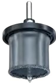
Holesaw, tungsten carbide gritted, complete with arbor and pilot drill, precision tube, coated with special tungsten carbide grit, high temperature brazed, for aerated concrete blocks, masonry, tiles, ceramics, natural stone, lightweight building materials, plasterboard and plastics, for installers, eg. switches and sockets, water pipes.
