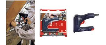
Electronic tacker TACKERTRONIX TT 14, extra high power, safety lever prevents accidental discharge, 220V/50/60 Hz supply, double insulated, radio/TV suppressed, 20 strokes/ min, for type 53 staples up to 14 mm, and type 55 brads up to 16 mm
