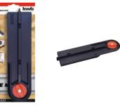
The sturdy angle fence fits all LINE MASTER precision rules. Angles can be set from 30 to 150 degrees in 15 degree steps. The retractable fin underneath allows use as an angle guide on the face of the workpiece or as a rip fence against the edge of the workpiece.
