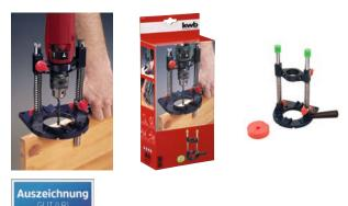
Drilling and milling attachment, for drills with 43 mm Euro-collar, two columns can swivel 90-45 degrees, for controlled drilling to exact depths or angles, continuous depth adjustment, exact control for serial drilling in lines, integral V-groove for securely holding curved workpieces.
