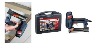
Electronic tacker TACKERTRONIX TT 26, professional tool in a plastic case, extra high power, safety lever prevents accidental discharge, 220V/50/60 Hz supply, double insulated, radio/TV suppressed, 20 strokes/min, for type 53 staples up to 26 mm, and type 55 brads up to 25 mm.
