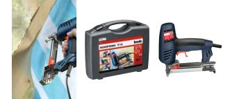
Electronic tacker TACKERTRONIX TT 18, professional tool in a plastic case, extra high power, safety lever prevents accidental discharge, 220V/50/60 Hz supply, double insulated, radio/TV suppressed, 20 strokes/min, for type 53 staples up to 20 mm, and type 55 brads up to 19 mm.
